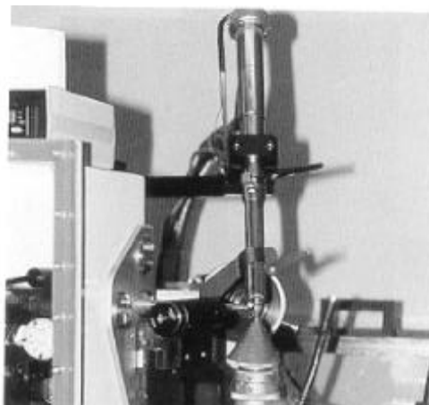
Fig 3. The position of the X-stream™ nozzle with respect to the goniometer as installed at UGA. The angle between the X-ray collimator and the nozzle is approximately 80° while the angle between the nozzle and the phi axis of the goniometer is approximately 150°. With this arrangement, ice formation has not been observed even during the humid Georgia summers.
