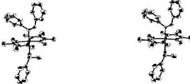
Fig. 2 Measurement with MoK $\alpha$  X-rays (cobaloxime complex).
