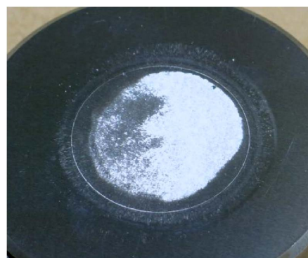
Fig. 11. Titanium oxide powder stuck to die after pelletization
