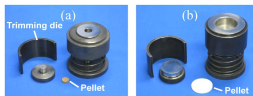
Fig. 5. Sample preparation with cylinder type dies.
