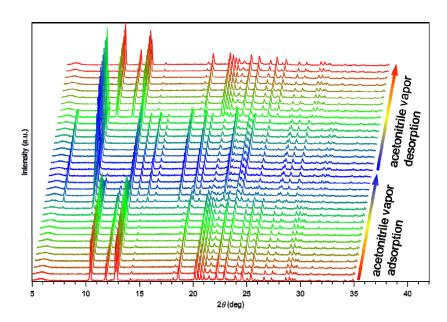
Powder diffraction patterns were measured by changing the vapor concentration of acetonitrile. The diffraction pattern of **1a** turned to that of **2** when the acetonitrile vapor concentration increased. When decreasing the vapor concentration, the diffraction pattern reverted to that of **1a**. Neither amorphous nor crystalline phases other than **1a** and **2** were observed, which indicates the transitions **1a** to **2** and **2** to **1a** occurred crystal-to-crystal.
