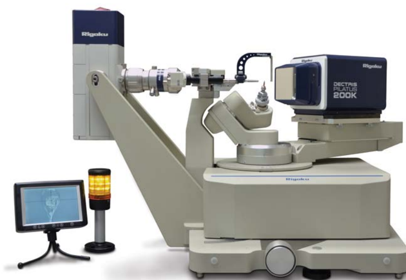
Figure 6. Compact HomeLab™ including PILATUS 200K HPAD
