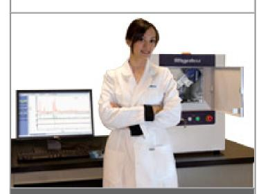
Benchtop X-ray diffraction (XRD) instrument
