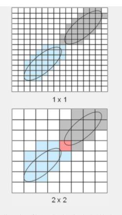
Illustration of how collecting data in 1x1 binning mode can help resolve diffraction spots.
