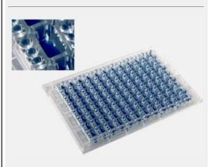
New CrystalMation<sup>TM</sup> Intelli-Plate<sup>TM</sup> 96-3 well crystallization plate that is optically clear, UVtransmissible, with low birefringence properties.
