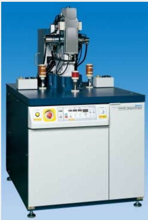
FR-E+ DW SuperBright dual wavelength rotating anode X-ray generator.
