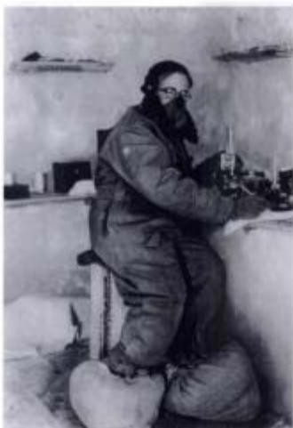
Fig. 123. The author with his polarizing microscope in his ice laboratory on the Jurglaupoch. The sponges over his nose and mouth served to prevent his breath fogging the eye-piece. The logs filled with hay kept his feet warm.
