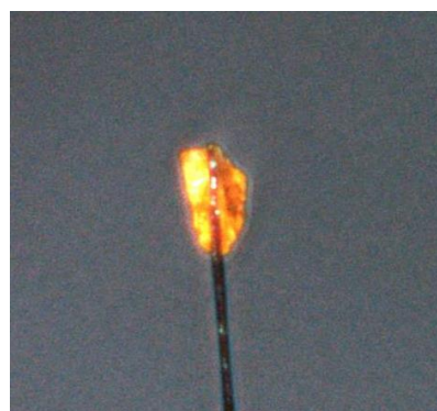
Figure 1. Crystal sample \mu (Ag) value of 47.5 mm -1 (0.10 x 0.08 x 0.03 mm)
