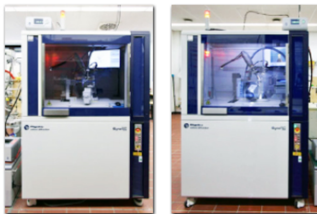
Left: Cu XtaLAB Synergy-S, right: Mo XtaLAB Synergy-S, both with 800 Series Cryostream systems. Not shown is an Xcalibur with an Eos detector.
